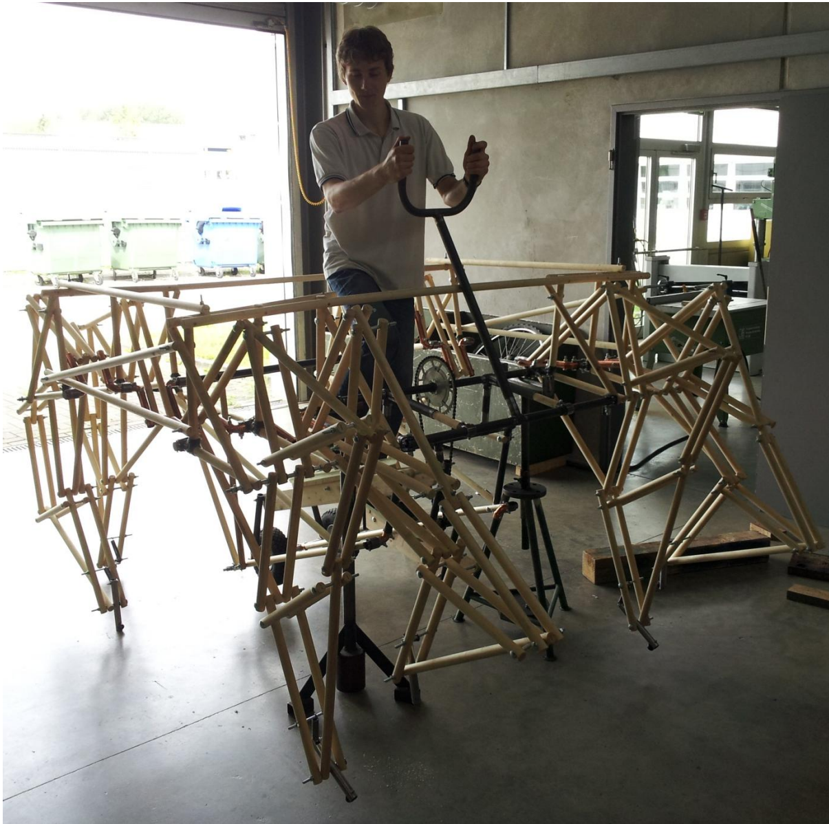
Illustration 12: Functional test with the jacked walking machine
