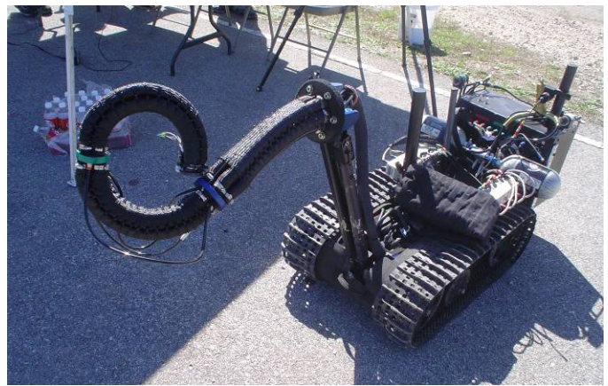
Fig. 7. OctArm V mounted on Foster-Miller TALON system.
