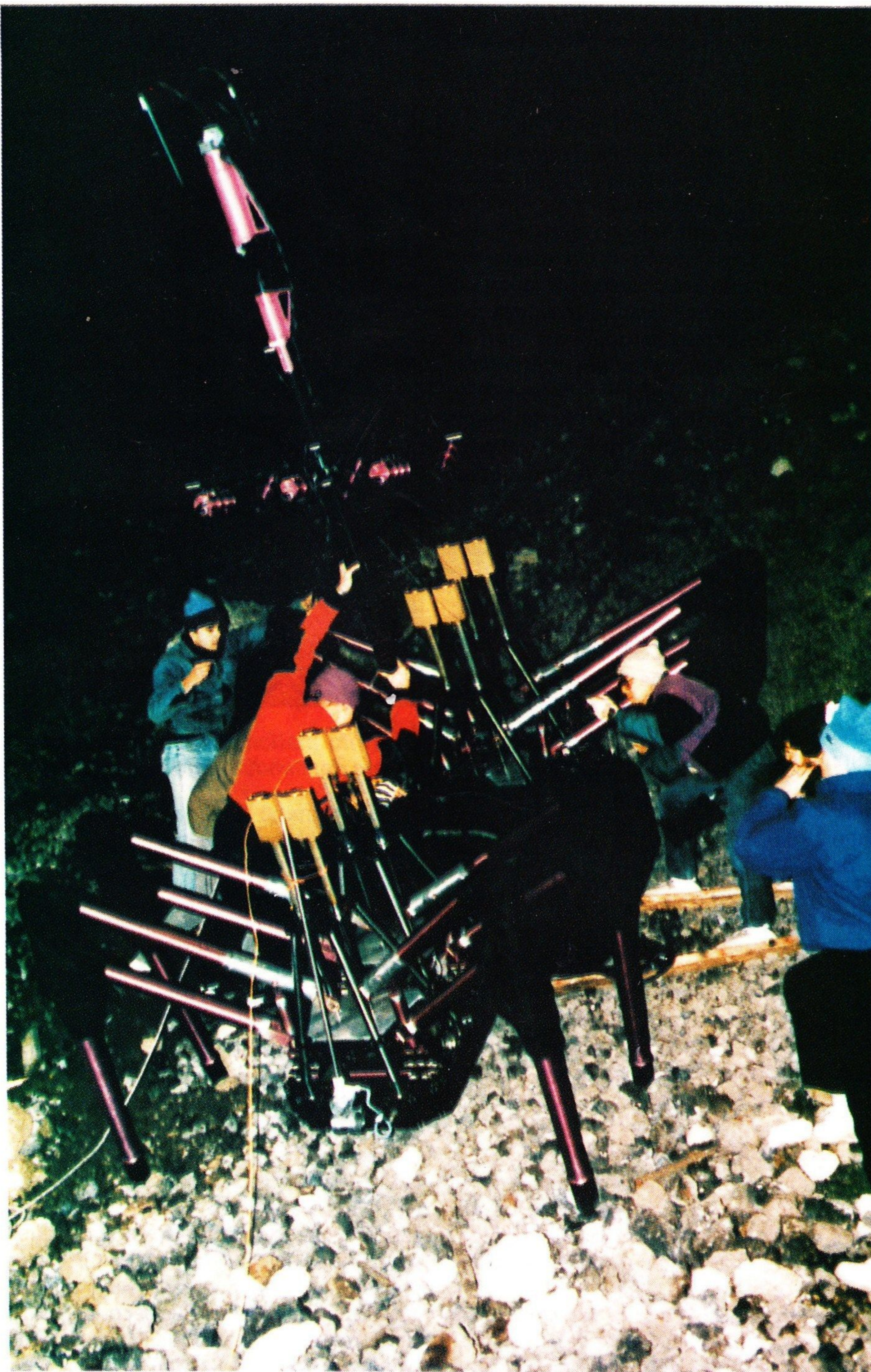
This photo shows the Dante robot making a test climb up a slag pile at Carnegie Mellon University, Pittsburgh, PA, in preparation for its Antarctic expedition. Our rather dramatic lead photograph is a screen shot showing the Dante robot in place on the rim of the crater ready for its descent into the Mount Erebus volcano.
