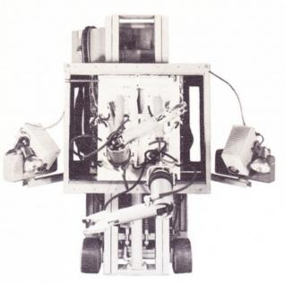
MOBOT Mark I was produced for a government contractor for handling radioactive materials in areas where radiation is too high for humans. It handles weights in the 150 pound class and operates up to 200 feet from the operator. It is mounted on a standard forklift truck for convenience and economy.
