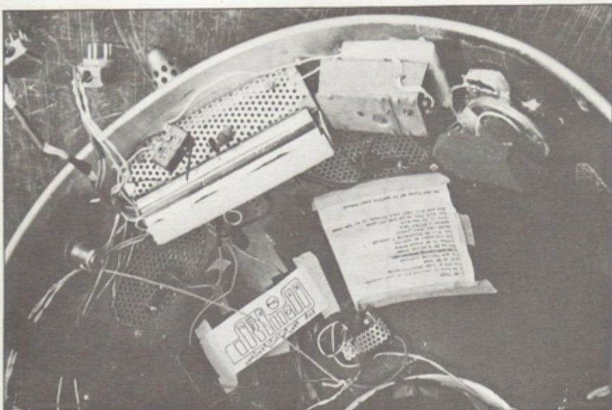
Interior of robot's head is a maze of wires. Note the socket plugs for easy removal of head and the script taped at eye level.
