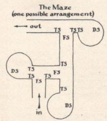
Mouse maze showing location of sensing switches (trolley omitted)
