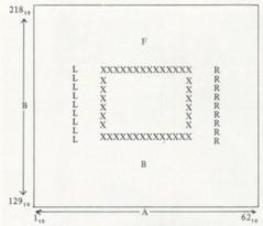
Within the square outlined by the X's, the robot will stop. The cursor must be moved close to the "F" or "B" for motion to begin. With "L" and "R", it is sufficient for the cursor to be behind the line of L's or R's, and not above or below the ending L's or R's.
