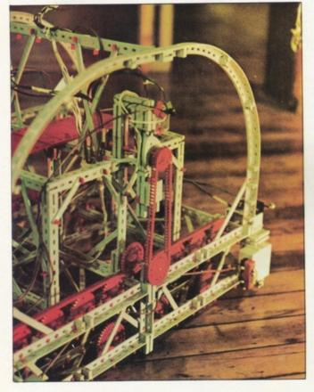
port. By sending ASCII characters to the interface, followed by an execute character, the relays change position, and power is supplied to specific motors in the robot.
